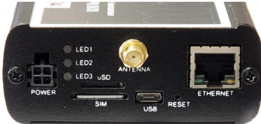
1. **Mount** a 2G/3G or 4G or an LTE 450/CDMA 450 **SMA antenna** to the **Antenna** titled SMA-M interface (according to the module/router type).
