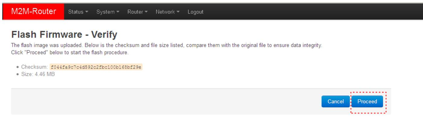
4. Then the next message appears on the screen in the browser. Then the refresh method has started, while the **LED2** and **LED3** is continuously lighting by **red**.
