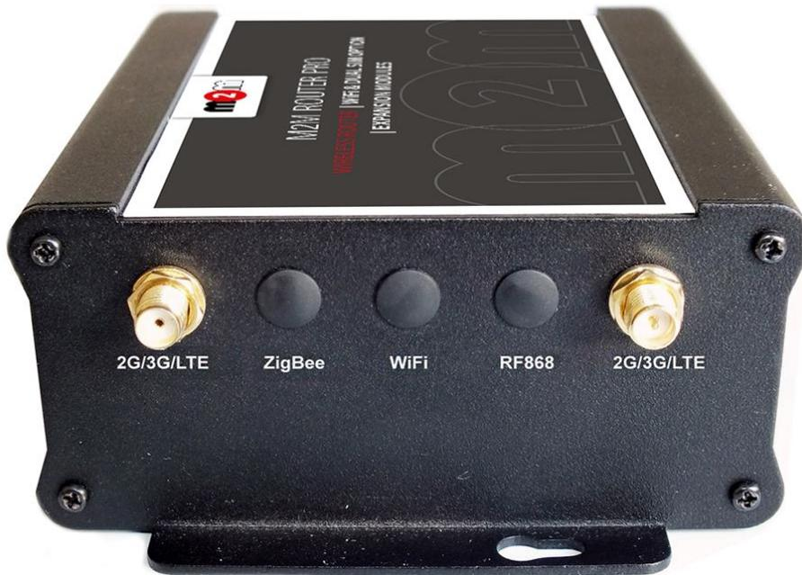
1. **Mount** a 2G/3G or two LTE **SMA antenna** – according to the module type - to one of the **Antenna** titled SMA-M interfaces (in case of LTE module all the two antenna must be mounted).
