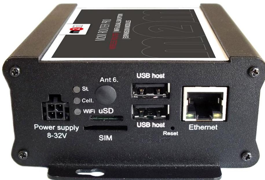
3. **Insert an activated data SIM card** to the SIM holder, placed the chip-side up and the cutted edge towards to inside and push until it sleeves.
